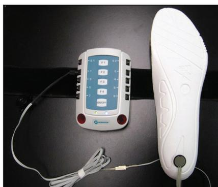
**FIGURE 1.** Audio biofeedback device and force transducer affixed to the rearfoot area of the shoe insole.
